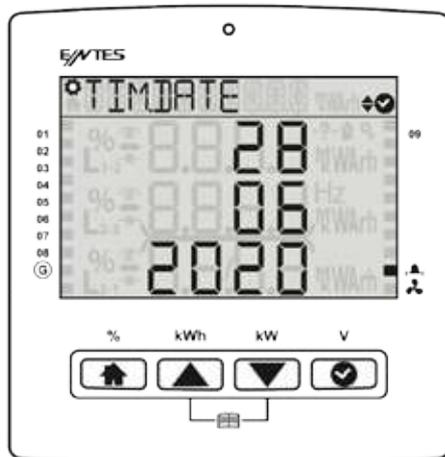
**3.1.6.3 Time** The user can set the current time on these screens. The change will be saved on the system without asking for conformation.
