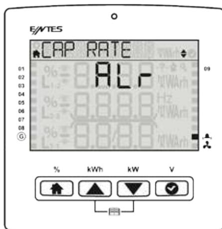
This screen shows that the inductive rate exceed's the warning limit.
