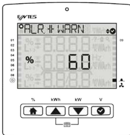
**3.1.5.8 Contactor Service Life Warning** This warning occurs when the rate of the switching count life exceeds the ratio set by the user. (Default value is 50.000 switching)
