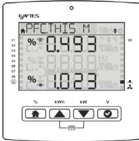
**3.3.1 Power factor correction Today** It is the menu where you can display the total inductive power factor correction rate, capacitive power factor correction rate values for today.
