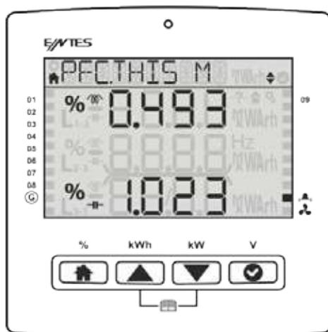
**3.3.5 Power factor correction Last Month** It is the menu where you can display the total inductive power factor correction rate, capacitive power factor correction rate and active .
