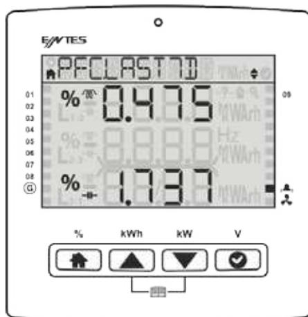
**3.3.4 Power factor correction This Month** It is the menu where you can display the total inductive power factor correction rate, capacitive power factor correction rate.
