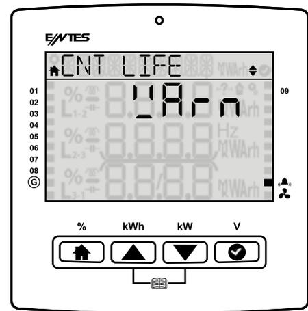
This message shows that the capacity loss of your capacitor is exceed's the alarm, warning limit.
