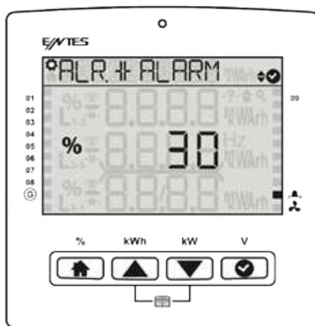
**3.1.5.7 Value Loss Warning** This warning occurs if the power of you capacitor is under the limit of your alarm. Ex: your original capacity is 100 kVAR. You set the alarm %30, when value becomes to 30 kVAR it gives warning
