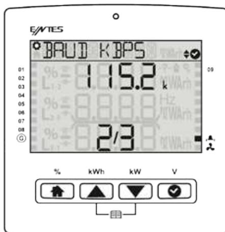
**Parity Bit:** The parity bit can be set to none, odd or even. The value of this parameter must be same as the value in the software you use to communicate with the product. Otherwise, you cannot communicate with the product.
