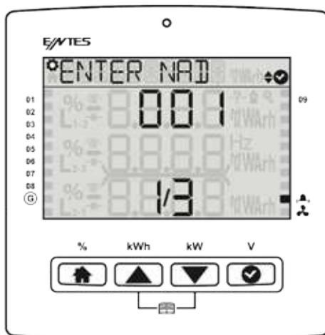
**Bit Rate:** This parameter can be set to one of the following values: 2400, 4800, 9600, 19200, 38400, 57600, 115200 or 256000 bps. The value of this parameter must be same as the value in the software you use to communicate with the product. Otherwise, you cannot communicate with the product.
