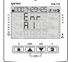
Press and hold the DOWN direction key for 2 seconds to go to the total power menu.
