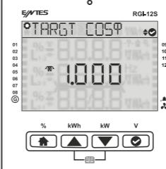
Enter the reference step and press OK. (Reference step must be 3-phase capacitor.)
