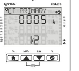
Enter the secondary value of the current transformer and press OK.
