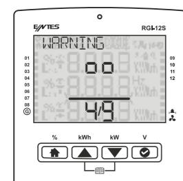
Notification LED of the device will light in Red. If the notification mode of the device is Red, this means that there is an alarm situation related to your system. You can press any key on your device to see the alarms. If you press OK, you can delay the alarm displayed. Press OK.
