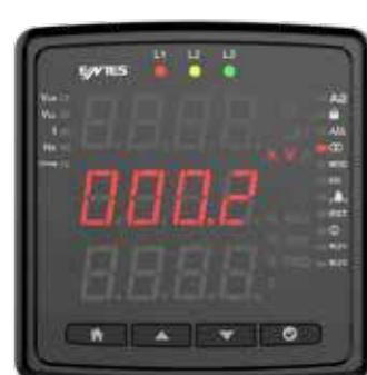
Press for the secondary value of the voltage transformer.
