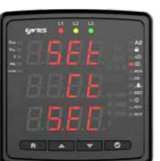
Enter the secondary value of the current transformer with buttons. Press buttons and choose the settings.
