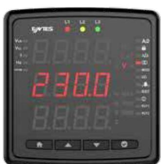
Press for the primary value of the current transformer with buttons.
