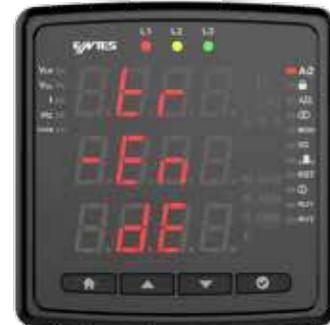
Press for the Voltage transformer settings
