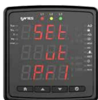
Enter the primary value with buttons of the voltage transformer.
