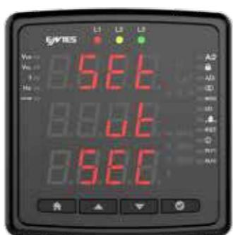
Enter the secondary with buttons value of the voltage transformer.
