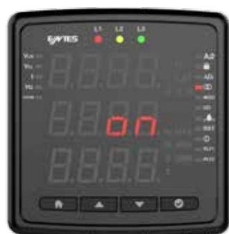
Press for the primary value of the voltage transformer.
