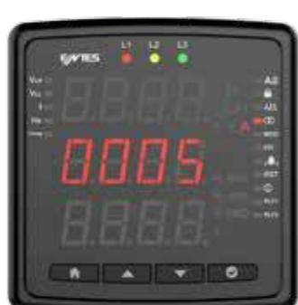
Press for the secondary value of the current transformer.
