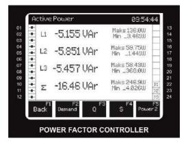
This screen displays active powers in phases, minimum and maximum values of these values, total active power, and minimum and maximum value of this value. If you press "Talep" (Demand) on this screen, the active power demand table will be displayed.
