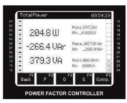
This screen displays total active, total reactive and total apparent powers, and minimum and maximum values of these powers.
