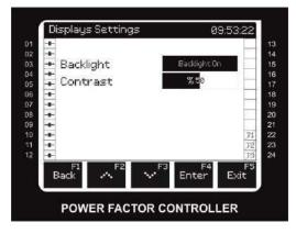
It is the screen where the user adjusts the contrast and light of the screen.
