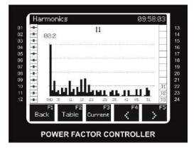
If you press the Harmonik (Harmonics) button on the Current Screen, all harmonics up to the 51st harmonic for I1 will be shown in bars. You can switch between currents using F4 and F5 keys.
