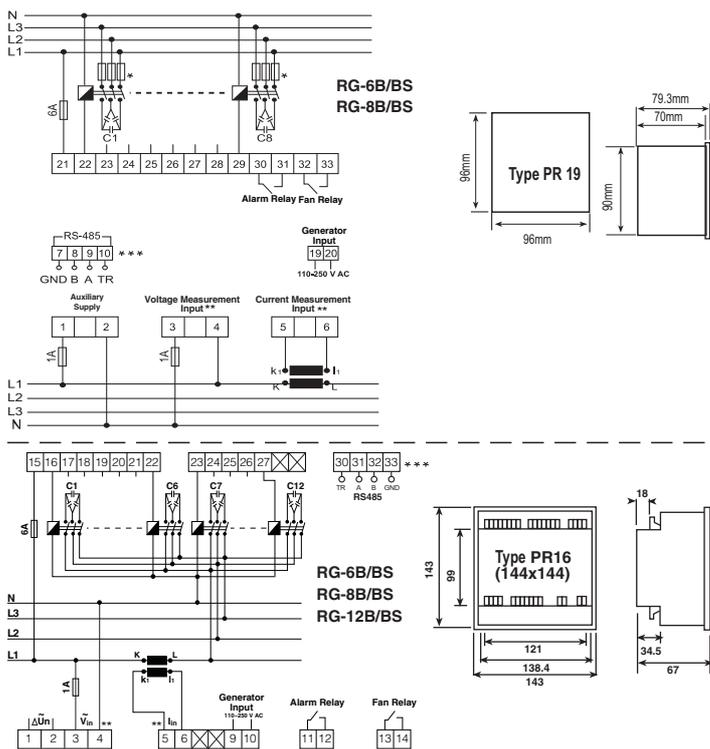
\* Current value of 3-Fuses, which are connected to protect the capacitors, is chosen according to the nominal current value of capacitors.
