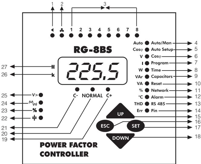
**NOTE:** Icon explanations are the same for type PR-19 and PR-16 models. The figure above shows the front panel of PR-19 RG-B/BS 08. The step numbers of the device shown with number 3 will change according to the model number.
