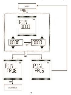
Basic settings map is shown below. There are two main submenus as function selection and display settings.
