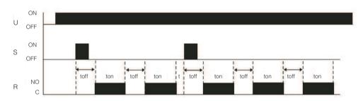
12.Adjustable ON Delay by external trigger leading edge
