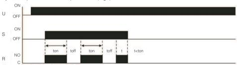
**9. Flasher / Start by external trigger leading edge / Relay OFF start** Function is similar to the ON Start version (function 8) with the exception that the output relay starts as passive.
