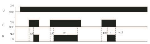
13.Adjustable and Resettable ON Delay Pulse by external trigger leading edge This function is controlled by start input after suply voltage is applied. The cycle starts with adjustable "toff" delay time after a pulse is created at the Start Input. At the end of delay time, output relay is activated and remain activated during "ton" time. If a re-trigger pulse occurs during "toff" time, elapsed time is reset and "toff" counting is restarted.
