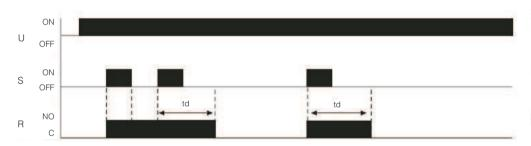
**16.** Adjustable OFF Delay Pulse by External Trigger Falling Edge Re-trigger This function is controlled by start input after supply voltage is applied. With the falling edge of the Start Input, output relay is activated and "td" time starts. After "td" time, the output relay is deactivated and stays that way until another pulse is applied to the Start Input. If another pulse is applied during "td" time, function is reset.
