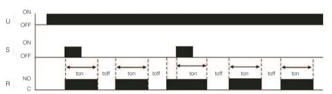
11. Flasher / Start by external edge - retrigger / Relay OFF start
