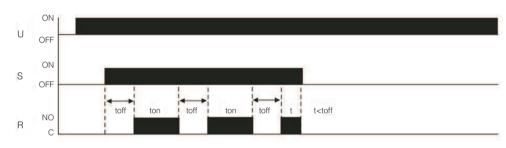
10. Flasher / Start by external edge - retrigger / Relay ON start
