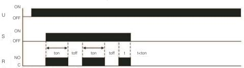
**9. Flasher / Start by external trigger leading edge / Relay OFF start**Function is similar to the ON Start version (function 8) with the exception that the output relay starts as passive.
