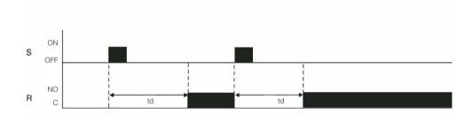
3. Off Delay / Start by external trigger trailing edge
