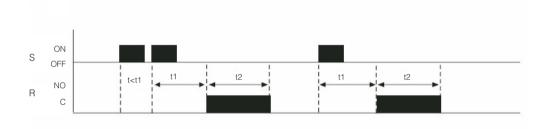
**14. Adjustable OFF Delay Pulse by External Trigger Leading Edge**This function is controlled by start input. With the leading edge of the external trigger, output relay is activated and remain on during **"td"**.
