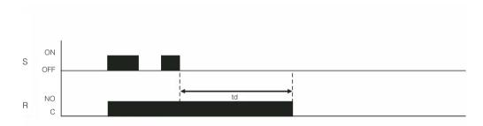
**4.** Symmetric Flasher / Start by external trigger leading edge / Relay ON start
